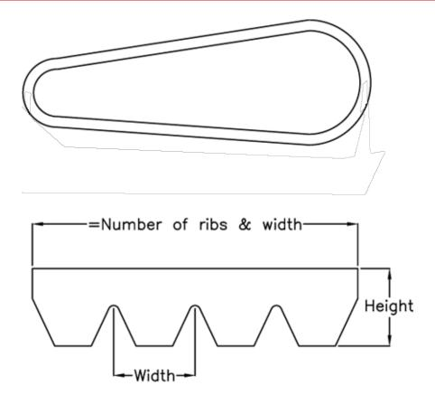
$\begin{aligned} & \text{Datum Llength} = 2324 \\ & \text{Height} & = 9.5 \\ & \text{Number of ribs} = 12 \\ & \text{Pitch} & = 4.7 \end{aligned}$
